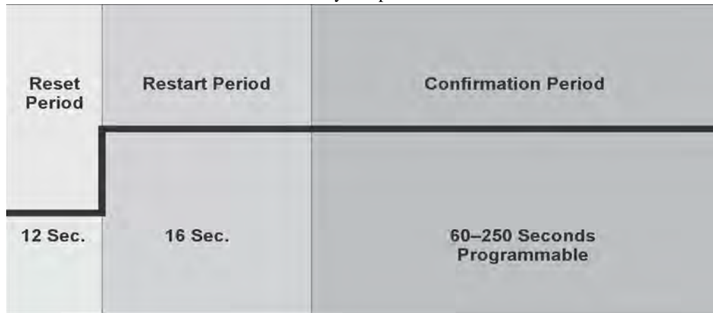
Figure 10.7 Smoke Verification Cycle
